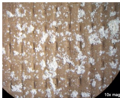
The bare mesh-backed tile and its rear face have been protected by a primer coat (WPM368) and bonded with X77 to concrete. The sample was immersed in water for several months, and the coating has protected the surface.
