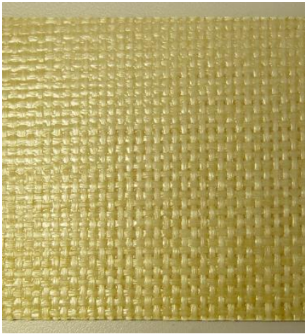
Mesh-backed tile with the mesh fully embedded in resin. Epoxy resins are difficult to bond to, while C-class tile adhesives can attack polyester resins.
