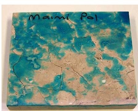
An example of a stone tile with significant potential for moisture marking
