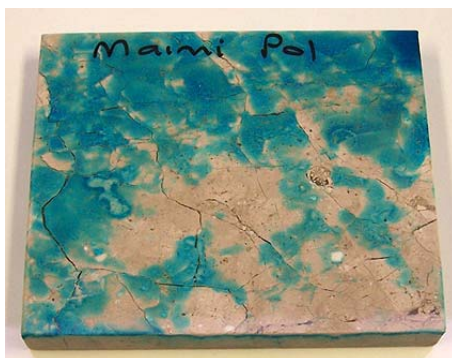
An example of a stone tile with significant potential for moisture marking
