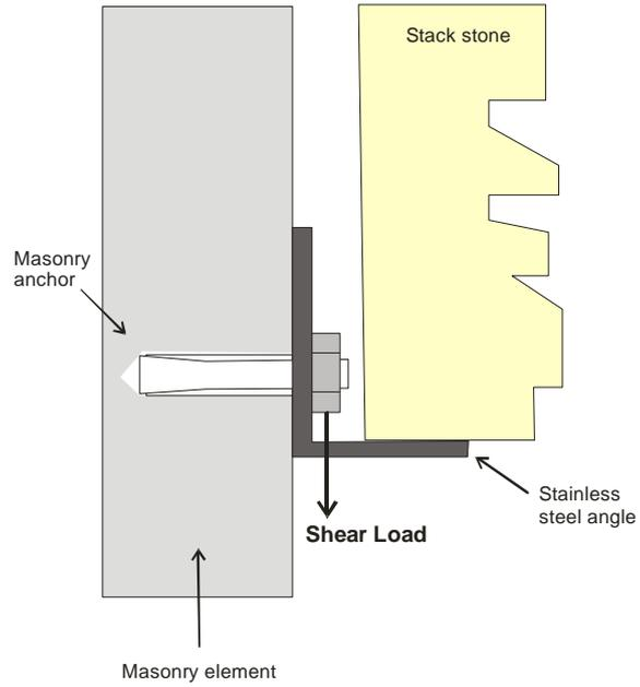
1b) Shear load exerted on the fastener by the cladding. Fasteners with too low a load rating may bend or shear off.
